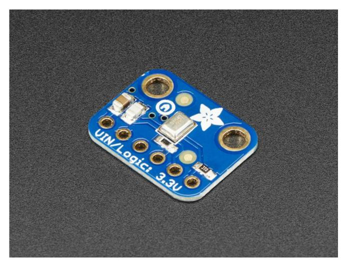
For many microcontrollers, adding audio input is easy with one of our analog microphone breakouts (http://adafru.it/1063). But as you get to bigger and better microcontrollers and microcomputers, you'll find that you don't always have an analog input, or maybe you want to avoid the noise that can seep in with an analog mic system. Once you get past 8-bit micros, you will often find an I2S peripheral, that can take *digital audio data* in! That's where this I2S Microphone Breakout comes in.
